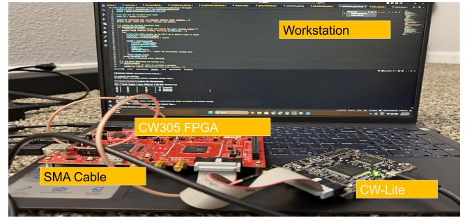
Figure 1. Experimental setup: ChipWhisperer CW305 FPGA target capturing global power via SMA
